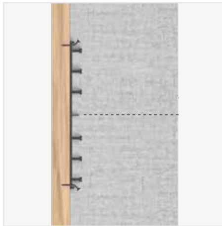
Wall-wall construction joint: Fastening to the formwork.
