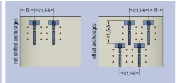
distance to the edge and the intermediate distances according to the drawing and the table must be complied with.
