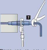
Hold the right-hand threaded female bar with a wrench and tighten the locknut to the specified torque using a torque wrench as for a male bar.
