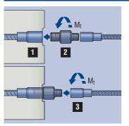
1 Concreted-in female bar with larger diameter.
