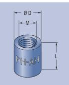
PFEIFER welding sockets are intended for areas in which steelwork and reinforced concrete parts are combined. By means of simply welding the PH-AH socket on, a connection can be made between the steelwork and the concrete part. The required thickness of the welded seam must be verified by the responsible engineer in accordance with DIN 18800.
