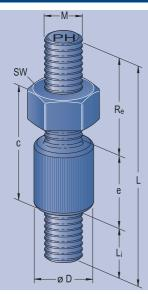
In the case that several bent bars have to be installed so close together that free turning of the bent bars is impossible, PFEIFER supplies the right-left threaded connecting bolt. The installation of nonrotating bars is hence possible without problems.
