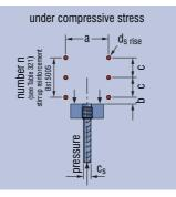
After the end anchoring plate has been screwed to the PFEIFER PH-A male bar in accordance with the approval, the bar can be installed together with the plate. Fundamentally, verification must be provided by the planner according to DIN 1992-1-1. The reinforcement shown Likewise, the specified minimum in the illustration on the left is merely a reinforcement that absorbs splitting forces from the end anchoring. A distinction must be made here between compressive and tensile forces.
