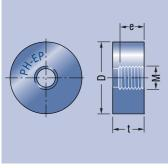
The PFEIFER PH-EP end anchoring plate allows users also to implement dynamic loads in accordance with DIN EN 1992-1-1. To this end the planner must determine the anchoring in accordance with the above-mentioned
