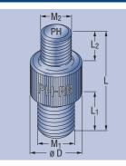
PFEIFER PH-RB reducing bolts are now available for the even more economical reduction of reinforcement cross-sections according to statical requirements. The reduction of diameters, which for example in the case of continuous columns often occurs in the upper floors
