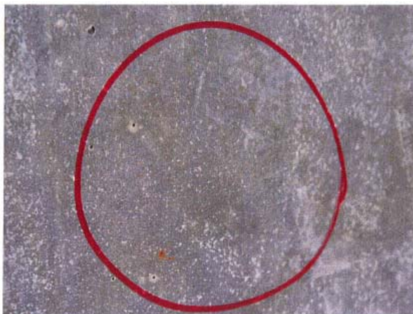
Fig. 4 Detail – undamaged outside surface of test specimen A – anchor 2
