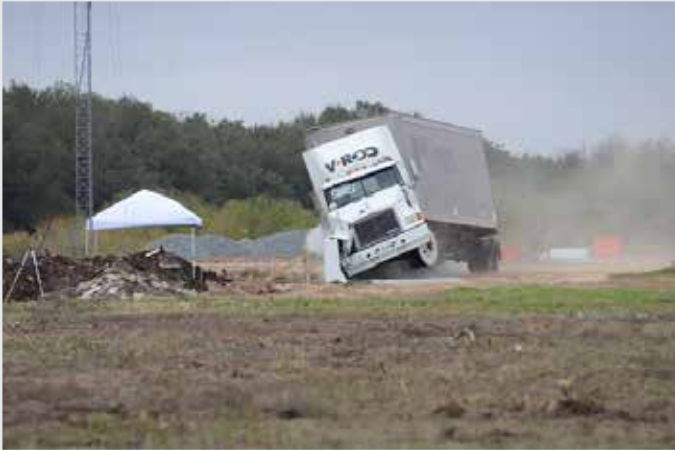
Impact testing with a 36 tonne truck at speed of 80km/h
