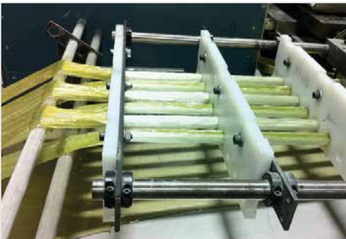
Manufacturing of FIBERNOX® V-ROD in the pultrusion process
