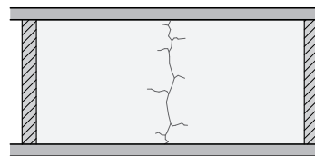
Cracks resulting from shrinkage and temperature fluctuations
