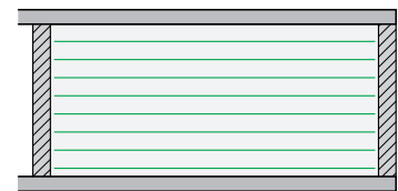
Cracks resulting from shrinkage and temperature fluctuations
